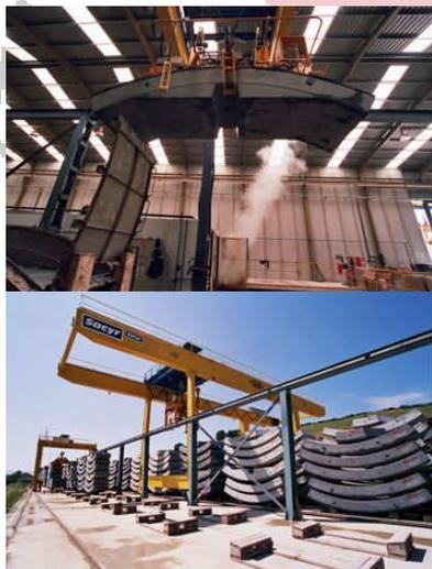
This factory, of French machinery, has been constructed exclusively for the manufacture of VOUSOIRS that are forming the ring that the tunnel boring machine is placing around the tunnel. Later, it injects fine gravels to the structure and a mortar that consolidates the hollow between the voussoir and the land. This is one of the main engineering jobs made in Málaga.
